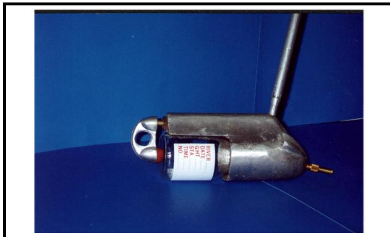
**Figure 3** DH-48 type depth integrating sampler
