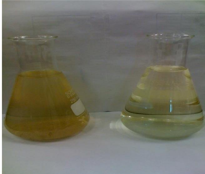
**Fig. 2:** Produced water before membrane filtration (left) compared with produced water after membrane filtration (right).
